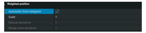
If the source does not provide a standard deviation value, it can manually be defined as a fixed value for the instrument, plus a range-dependant part.
