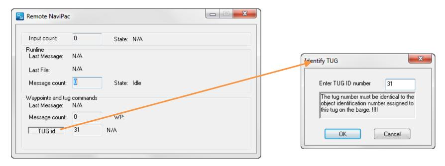
To receive the anchor pattern on the Tug, the Remote NaviPac window will be opened automatically when entering online mode. Click on the 'TUG id' text-box and the window to the right will open. Now insert the ID (31 for Tug 1 etc). NaviPac will remember this setting.
