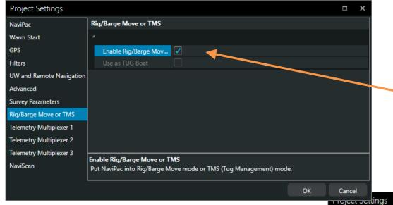
On the Barge, Rig/Barge mode must be enabled.
