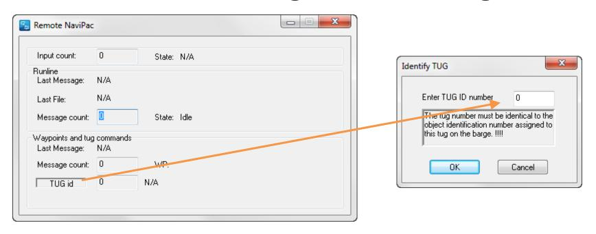
When in online mode, click on the 'TUG id' text-box and the window to the right will open. Now insert the ID (0 - telling that this is the barge). NaviPac will remember this setting. The window should never be closed, as it acts as interface between the NaviPac kernel (interpreter) and the TMS kernel (RigMon).
