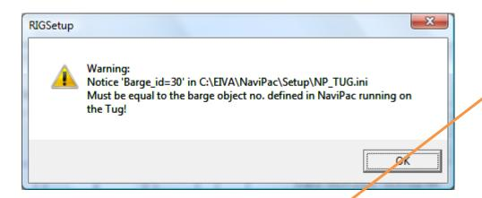
When saving the TUG Rigmove Setup file, the warning above is given.
