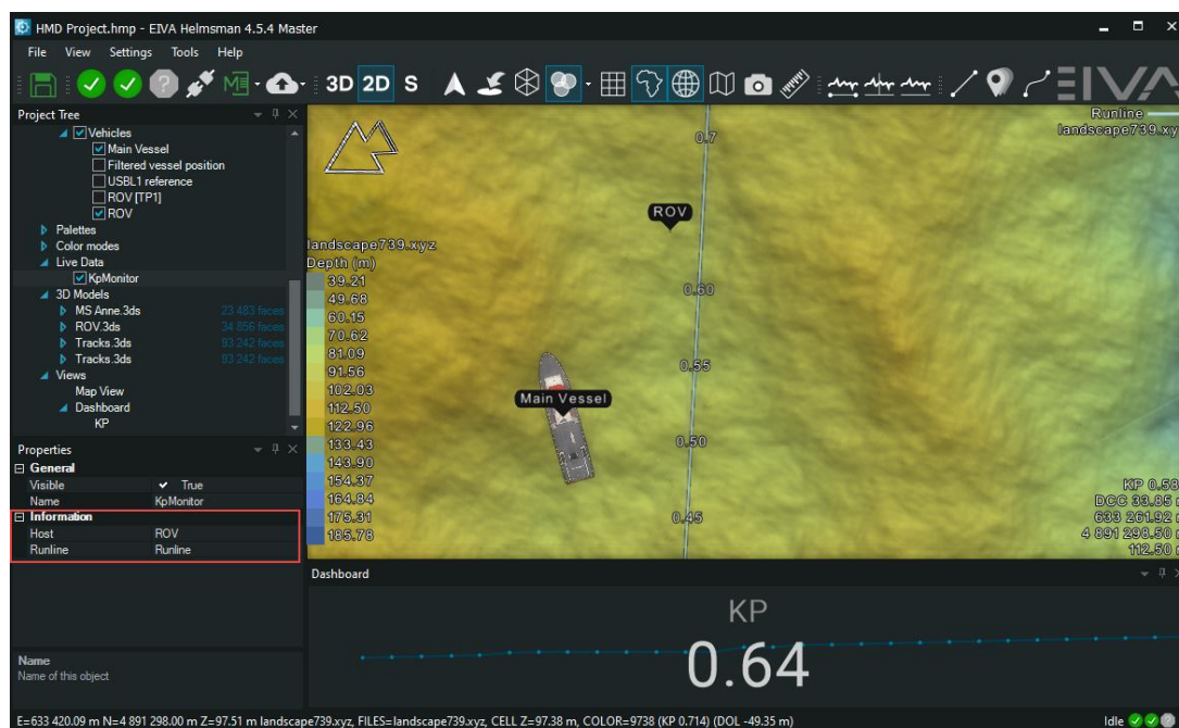
Figure 55 Kp for object displayed as Data View; the name, host and runline can be selected from the Properties Panel (red box)
