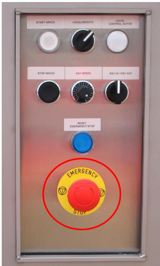
Figur 2 Electrical cabinet located on winch
