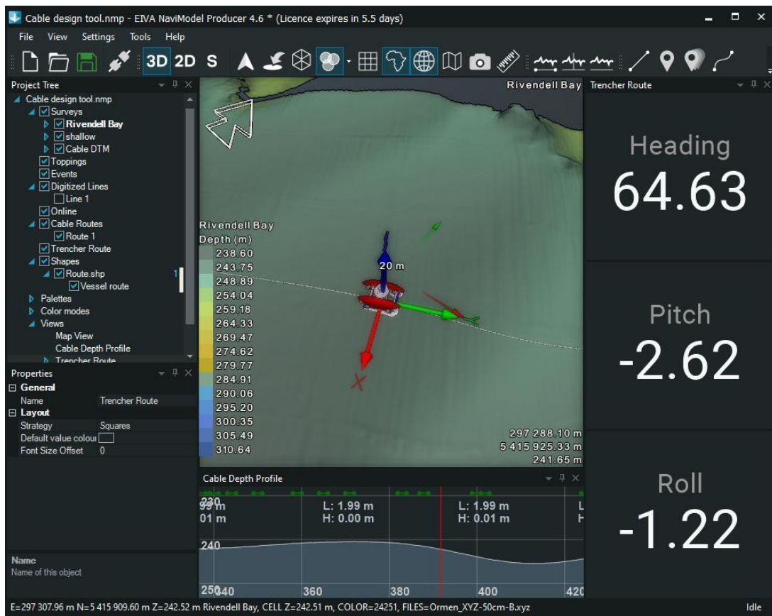
Figure 19 Dashboard showing Heading, Pitch, and Roll values
